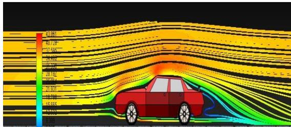
Fig.11: Flow trajectories showing velocity of flow over modified car model.
