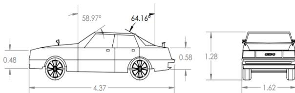
Fig.1: Schematic representation of the simple car (Linear distances are in meter and angles are in degree)
