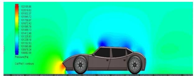
Fig.15: Pressure distribution over concept car model.
