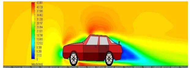
Fig. 9: Velocity distribution over modified car model
