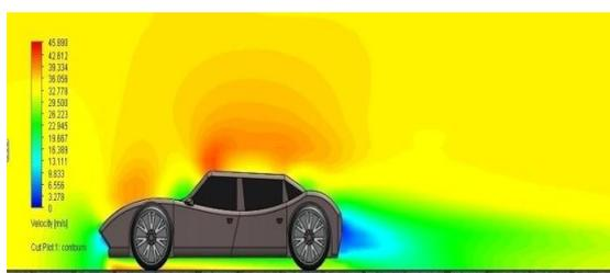
Fig.14: Velocity distribution over concept car model.
