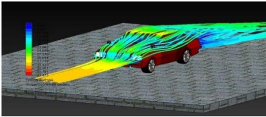
Fig.5: Flow Trajectories of the simple car.
