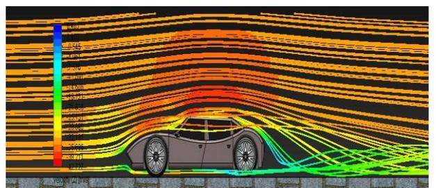
Fig.16: Flow trajectories showing velocity of flow over concept car model
