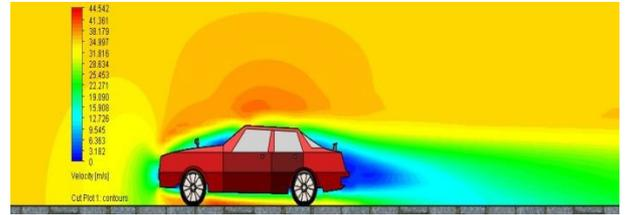
Fig. 3: Velocity distribution of Simple car model.
