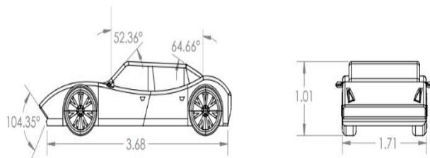
Fig.12: Schematic representation of concept car (Linear distances are in meter and angles are in degree)
