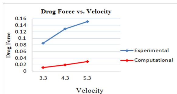
Fig.21: Experimental and computational drag force of concept car at different wind velocities.
