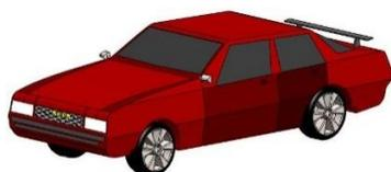
Fig.8: Three dimensional solid model of modified car. In the modified version of the simple car model, the sharp edge of the car is modified into fillet with concern in style and fashion to reduce the resistance of air. The targeted regions of the front is transformed by making smooth inclination so that the velocity can flow smoothly over the car. A remarkable modification is also accomplished in the sight glasses in the front of the car.
