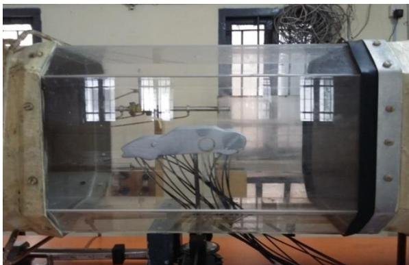
Fig.18: Wooden model inside conventional wind tunnel
