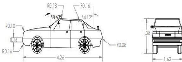
Fig.7: Schematic representation of the modified car (Linear distances are in meter and angles are in degree)
