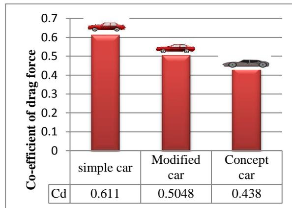
Fig.20: Computational of drag coefficients
