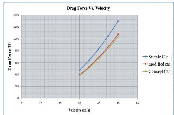
Fig.19: Variation of drag force with air velocity
