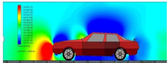
Fig.10: Pressure distribution over modified car model
