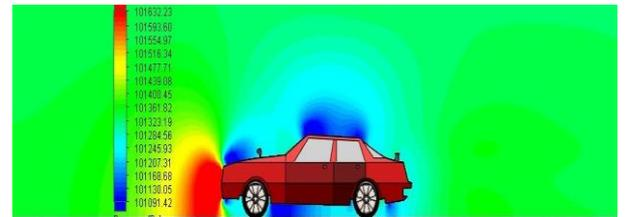
Fig.4: Pressure distribution of the simple car model
