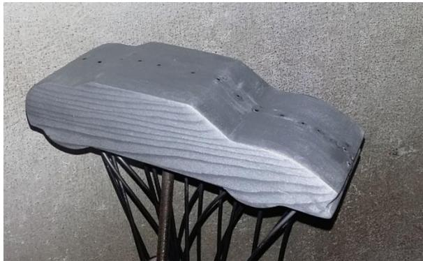
Fig.17: Wooden model of the concept car with pressure tapings.
